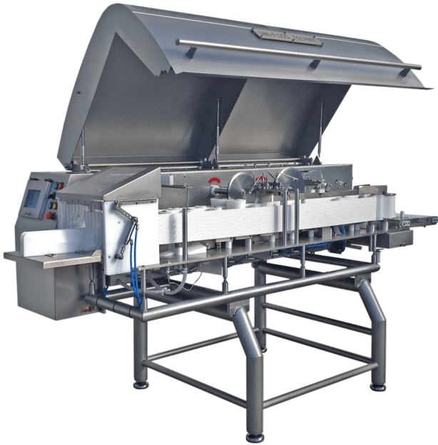
FR 9000 Filleting Machine for Salmon and Trout, for fish size 2-10 kg
