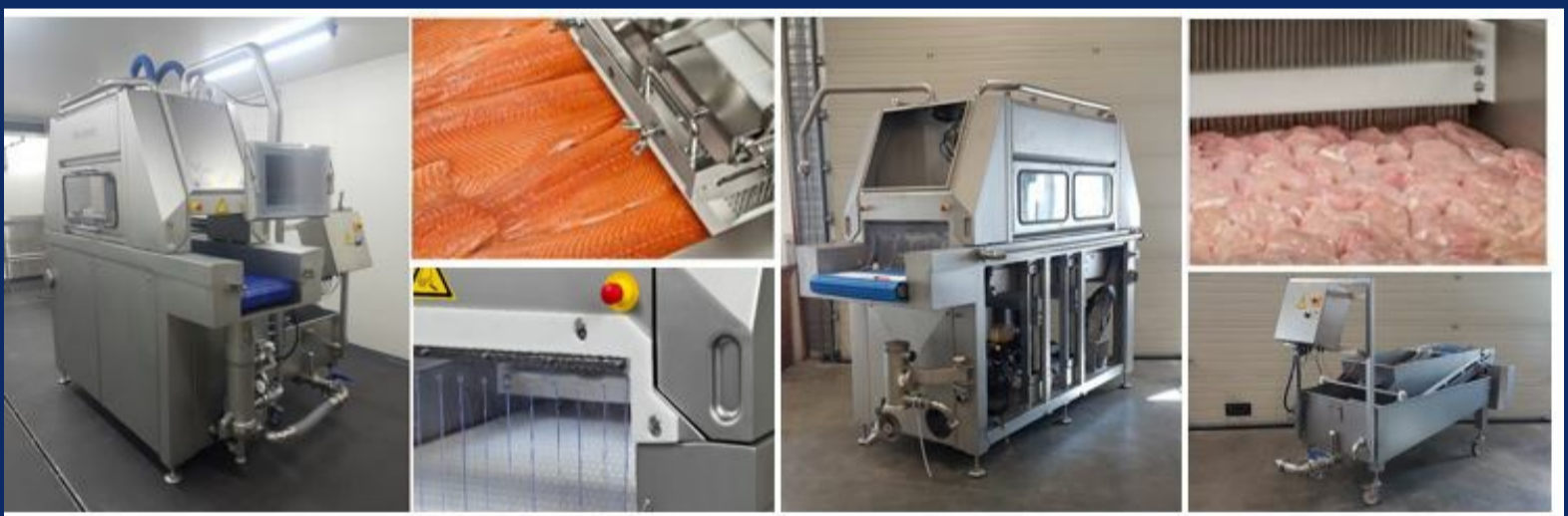
M3 enkelkops Pekelijector incl. FM 80 proteïne filter & CBF 500 bandfilter
