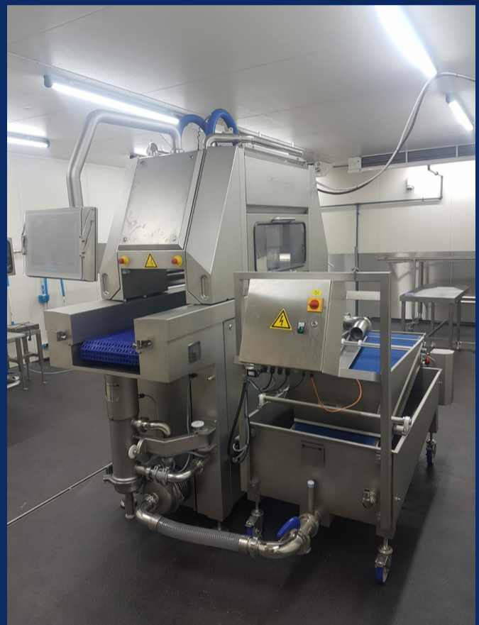
M3 enkelkops Pekelijector incl. FM 80 proteïne filter & CBF 500 bandfilter
