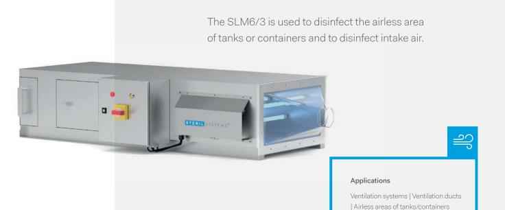
The SLM6/3 is used to guide air through three filter stages (G4, F7, H13) for treatment and filtration. Then the air is disinfected by the UV-C module, after which it is blown into the existing tank.
